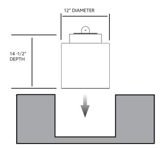
**Step 3.** Insert concrete cylinder and level with floor/pavers.
