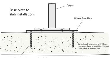
M10 concrete screw or dyna bolt minimum length 75mm
